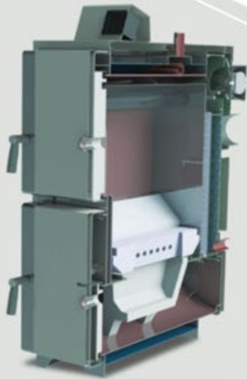
Cross Section of Ventum Boiler
